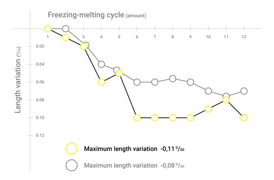
The change in the length of the specimen material in the frost resistance test after the freezing-melting cycle does not exceed 0.1 peri (0.01%). According to the German standard, up to 1 promil is allowed for the concrete. Therefore the StabilRoad is 100 X more efficient!
